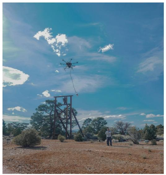
Drone with suspended magnetometer above the Golden Pipe shaft and headframe.
